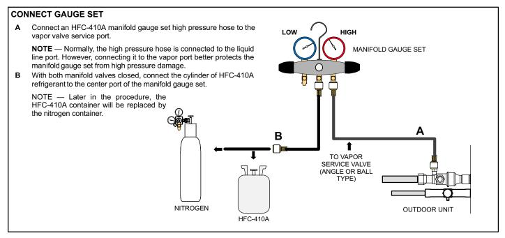
Figure 12. Manifold Gauge Set Connections for Leak Testing
